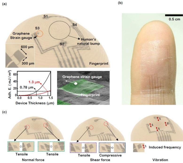
**Figure 1 a. Illustration of conformal graphene 3-axis sensor, calculated adhesion energy of the sensor as a function of the substrate's thickness and SEM image b. Photographs of a conformal 3-axis sensor. c. Illustration of operation principle related to the normal force, shear force and vibration.**
